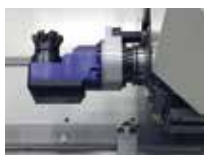
Hobbing of gear teeth (Flanx-Hob)
