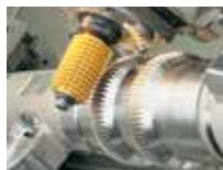
Hobbing of gear teeth (Flanx-Hob)
