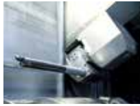
Drilling + ID boring
